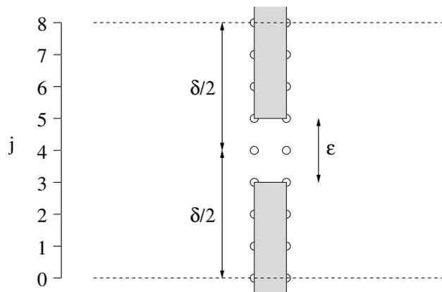
Figure 2: Insulating wall with holes, periodic boundary
