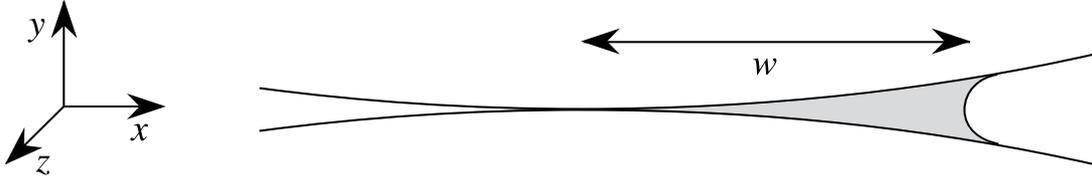
Making appropriate geometrical approximations, show that the cross-sectional area of fluid is proportional to  $w^3$  and that the curvature of the semicircular meniscus is proportional to  $w^{-2}$ . Find the constants of proportionality.
