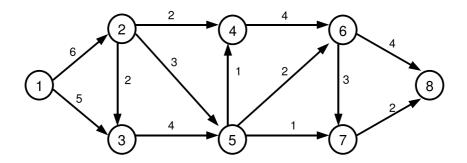
Here the number by each arc represents the capacity of that arc. What is the min-cut of this network?
