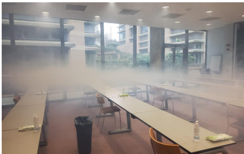
Figure 2: MR4 in December 2020. The external temperature was 5-8°C and the ventilation system had been running for over an hour. Artificial smoke, with a buoyancy comparable to breath, was released and became trapped in the breathing zone. (The inlet duct had been modified to deflect the airflow downwards.)
